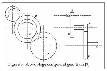
As in between a meshing pair a small gear is more prone to failure than larger gear when both are made of same material so here we will concentrate only on small gear for stress strength constraints [8].
